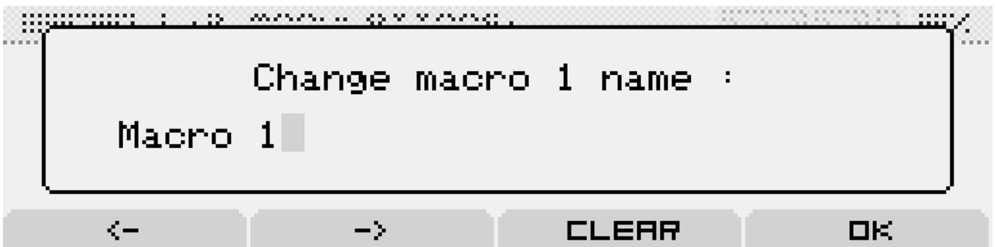
Here, you can enter a new name for the macro. Use the left and right arrows to move the cursor. The encoder allows you to change the letter or number at the cursor's position.
