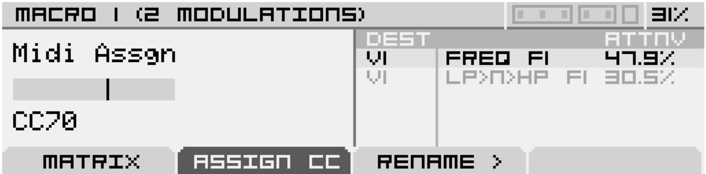
In the "ASSIGN CC" tab, the "Midi Assgn" parameter allows you to assign a MIDI Control Change from 1 to 119.
