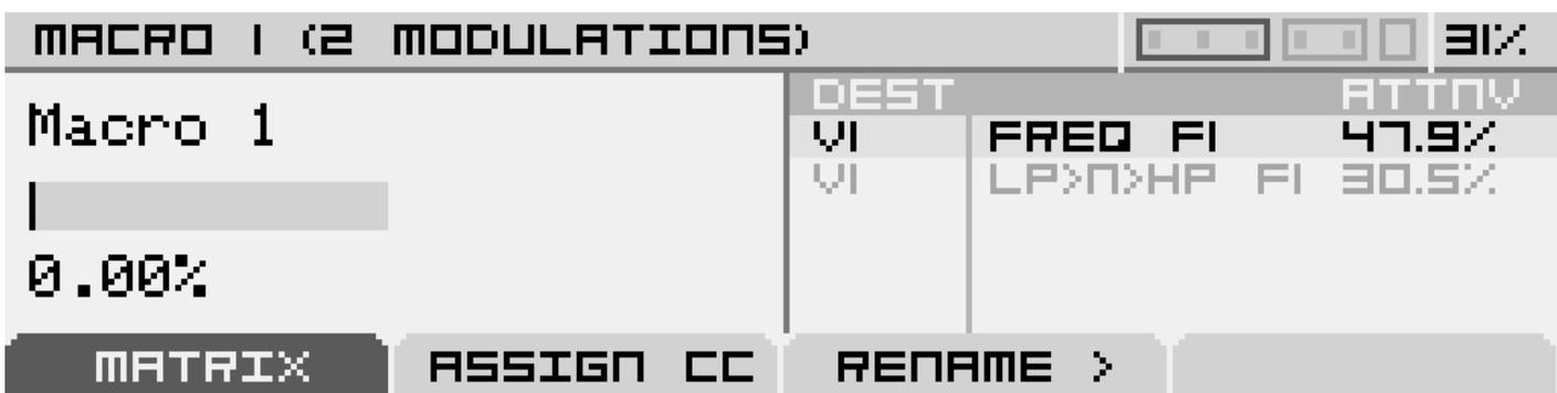
On this screen, you can adjust the macro's current value and view its modulation matrix. In this example, the macro controls two parameters: "Freq F1" and "LP>N>HP F1," with attenuverters set differently for each parameter.
