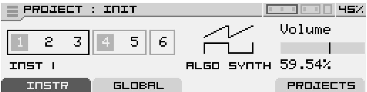
The project screen is the first screen displayed when the module is powered on. It provides an overview of the instruments and their voices. On this screen, you can create a new project, save it, load an existing one, and access all of Antigone's functionalities.
