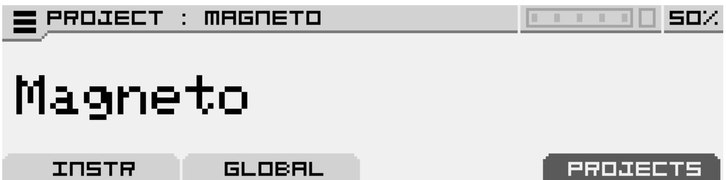
This tab allows you to quickly browse through saved projects in the current directory. Turn the encoder left or right to directly load the next or previous project.
