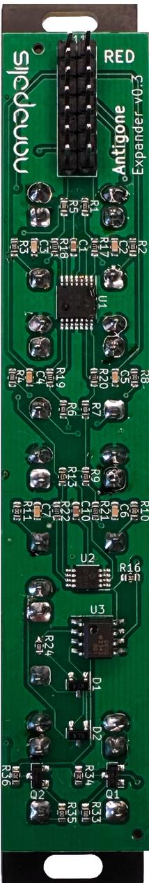
Warning ! The ribbon cable must be plugged in the right direction. There is a "RED" inscription on the PCB which indicates where the red stripe of the ribbon should be.
