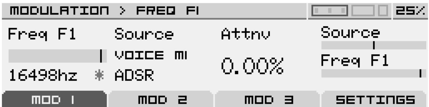
The modulation screen allows you to assign up to three internal or external modulations to a specific parameter on the module.
